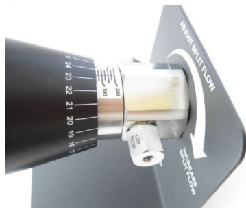
Inlet Port/Nut (replaceable filter is installed inside)
